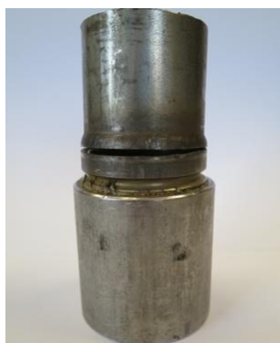
(e) Weld failure in riser pipe Source: Tony Beers.
