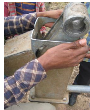
(d) Broken handle on Afridev pump in Malawi Source: Larry Bentley.
