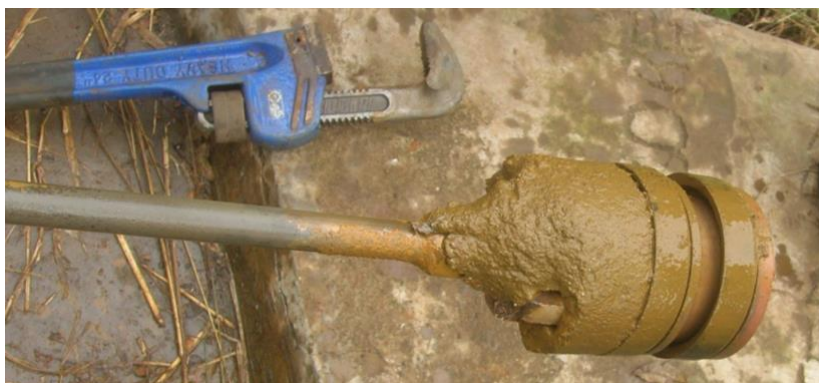
FIGURE 7 FOOT VALVE COVERED WITH DEBRIS FROM CORROSION Source: Larry Bentley.
