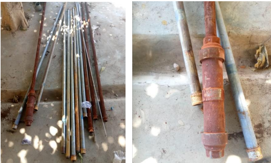
FIGURE A2.3 PHOTOGRAPHIC EVIDENCE OF RAPID HANDPUMP CORROSION IN KATSINA STATE, NIGERIA
