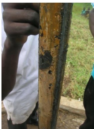
(a) Removal of pitted pipes within, Hoima District, Uganda, 2012 Source: Larry Bentley.
