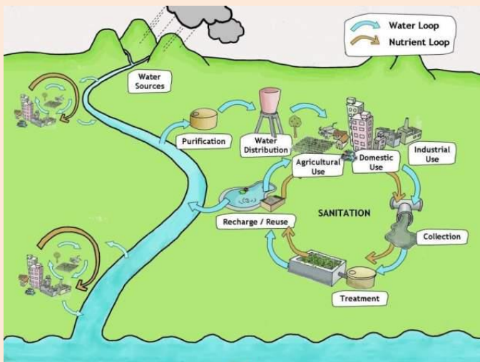
Figure (above): Using the water cycle for water supply ( www.sswm.info )
