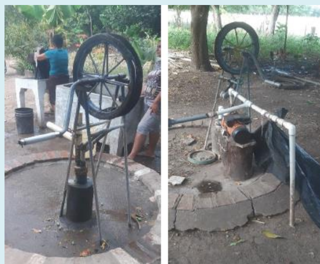
Figure 3: Left: A functioning original rope pump on a family well (shared by two households) used for human consumption, washing, bathing and irrigation of patio garden; Matapalo village, Villanueva. Right: An original rope pump no longer in use, replaced by an electric centrifugal pump; Aquespalapa village, Villanueva. Source: Briemberg (2022).
